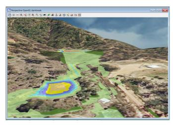
In this 12d Model movie, the centre of the dam collapses and the resulting flood wave with depth colouring is shown.
