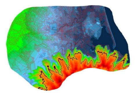
LiDAR using 12d Model coloured depth polygons illustrating changes in elevation
