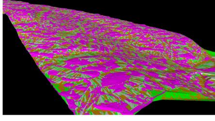
TINs made from ALS (magenta), ALS derived contours (grey), contour derived DTM (green) and filtered DTM (brown). Looking at the successive TINs in 12d Model like this allows visual comparison to see where and how averaging is taking effect. The 'patchwork guilt' appearance is good. It means the surfaces have been effectively averaged each time. Area with too much of one colour may need review or replacement with denser data.
