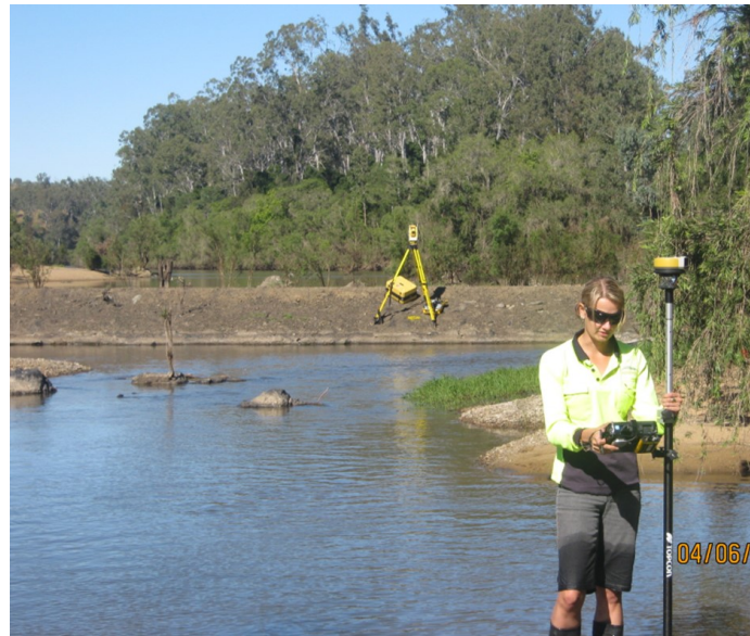
Survey field trials using Toughbooks with 12d Field and FDO technology. Wireless broadband allows direct connection back to ArcGIS servers.
