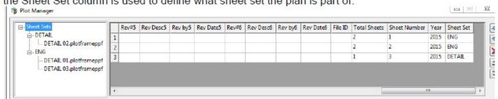
The sheet order can be changed by using the arrows to the right of the table. The sheets can be renumbered using the renumber button (Refer to 3.6.3).
